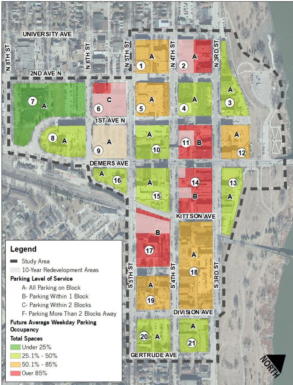
Figure 67: 10-Year Average Weekday Occupancy and Parking Level of Service for All Spaces Under the 10-Year Redevelopment Scenario
