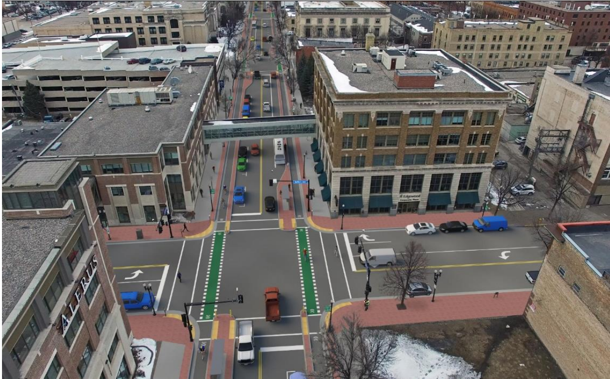
Figure 106: Example Protected Bicycle Lanes on 4th Street
